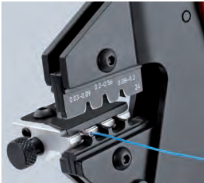
97 43 400 with crimping dies 97 49 24 and locator 97 49 93 for D-Sub plugs
