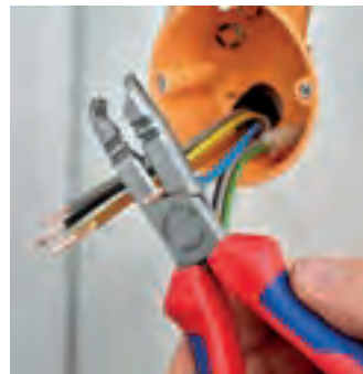
Cutting edges shortening of single wires
