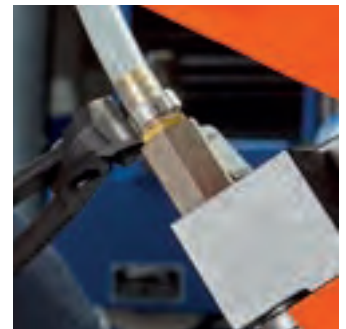
Sealing the hose connection on central lubrication
