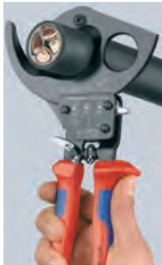
Ratchet principle and two-stage ratchet drive for easier cutting
