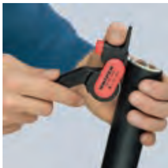
Setting the tool for longitudinal cut
