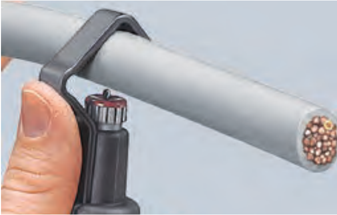
Setting the tool for circular cutting
