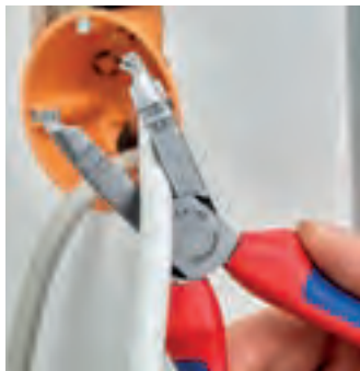
Cutting cable up to 13 mm diameter
