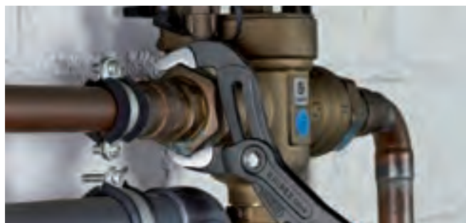
Teeth set against the direction of rotation have a self-locking effect and prevent slipping on the workpiece
