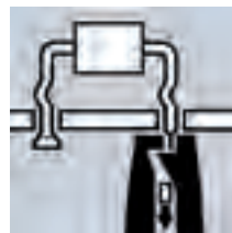
36 32 125 to crunch and cut wire at 1.6 mm length below the board
