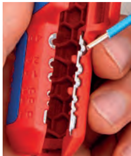
Stripping of single conductors
