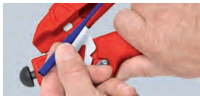
The assembly tool comes with three torpedo mandrels for the various cable cross-sections
