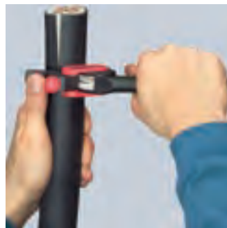
Turning the tool for circumferential cut
