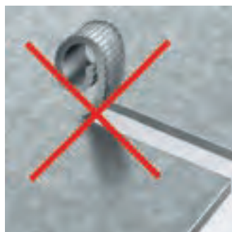
Notching without chip breaking
