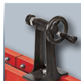
Tailstock with live spindle tip for securing and centering the workpiece, tool-free adjustable
