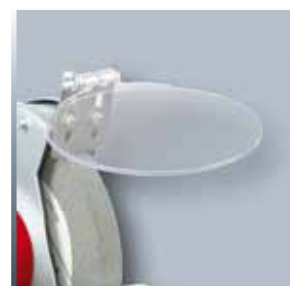
Adjustable spark guard window
