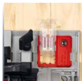
Additional marking of the sawing line
