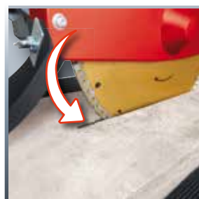
Plunge cutting function
