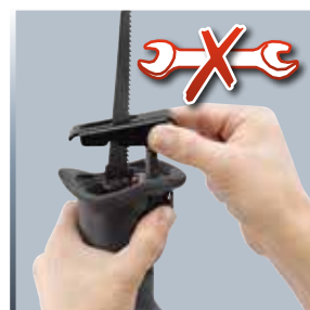
Toolless soleplate adjustment for optimum blade use
