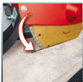
Plunge cutting function
