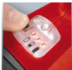
LED battery capacity indicator
