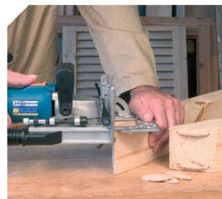
Stronger joints with No. 6 splines.
