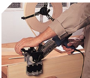
High precision and stability during edgebanding.
