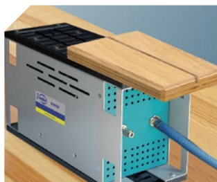
Small piece clamped on divisible suction plate.
