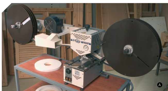
Easy access glue tank on top. The glue application system includes an easy, non-stick silicon roller.
