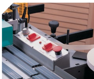
Safety control (STOP). Electronic temperature control.
