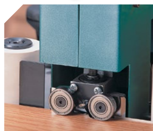
Power trimming unit: trimming both sides simultaneously.
