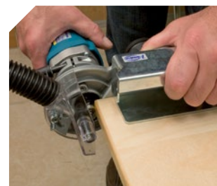
Precise guiding for corner trimming.
