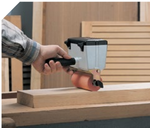
Gluing with vinyl (white) glues
