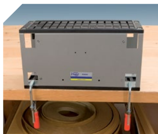
Small piece clamped on divisible suction plate.
