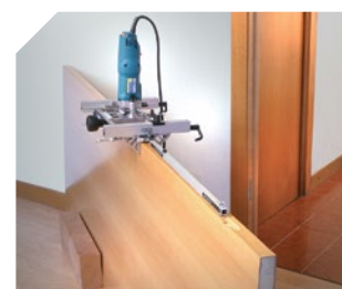
To make other recesses both on frames and doors it is not necessary to readjust the machine.
