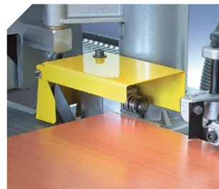
Front and rear flush cutting (tapes up to 2 mm thickness only).
