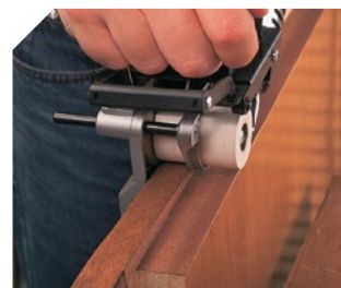
Banding the upper side of the lap.
