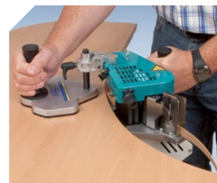
Easy to clamp on rough surfaces by clamping screws.
