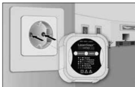
Plug the device into the socket. Make sure that the word TOP is at the top.
